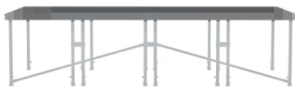
Arriostramiento a 2 metros con Bidas Dbles Braces at 2 metres with double Flanges
